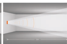
50m detection length @ 5m mounting height
